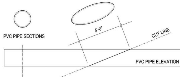
LOCATE CUT LINE BY MEASURING APPROX. LENGTH OF OVAL ALONG PIPE ELEVATION
